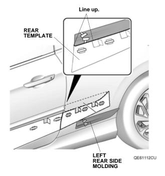
While applying light pressure to the left rear side molding, carefully remove the taped adhesive backings.
