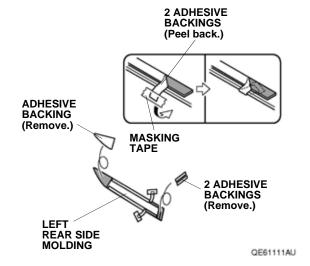
12. Line up the left rear side molding with the rear template, and attach it to the left rear panel as shown.
