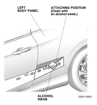
7. Peel back the adhesive backings and tape them to the front surface of the left front side molding. Remove the other adhesive backings.
