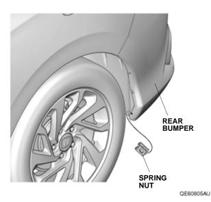
7. Secure the left rear splash guard with two self-tapping screws in the order shown below. NOTE: Make sure there is no gap between the left rear splash guard and the bumper. If there is a gap, loosen the self-tapping screws, hold the splash guard against the bumper, and retighten the self-tapping screws.
