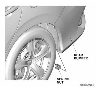
7. Secure the left rear splash guard with two self-tapping screws in the order shown below. NOTE: Make sure there are no gaps between the left rear splash guard and the bumper. If there is a gap, loosen the self-tapping screws, hold the splash guard against the bumper, and retighten the screws.
