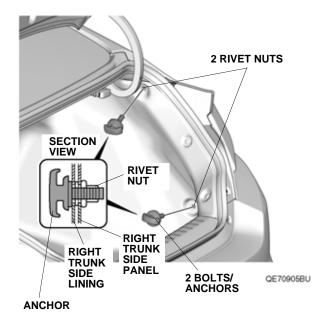
14. Install the cargo net to the anchors in the trunk.
