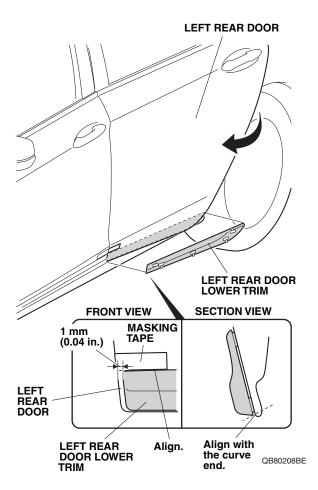
12. While applying light pressure against the trim, carefully remove the taped adhesive backings.
