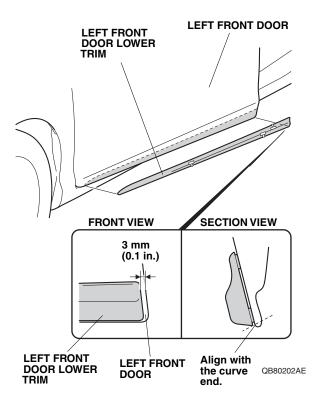
4. While applying light pressure against the trim, carefully remove the taped adhesive backings.
